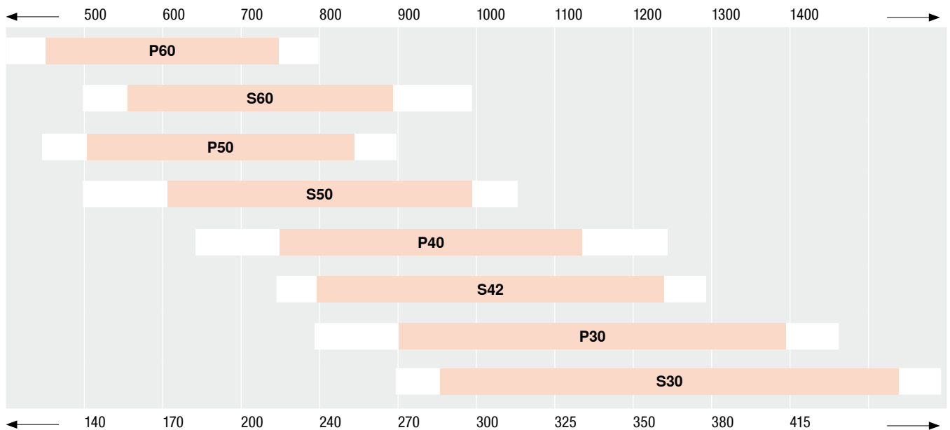
Recommended application range for support chamfers based on the BRINELL hardness of the steel material (HB)
